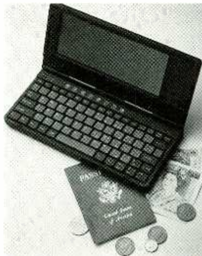
FIG. 1—ZEOS' $600 Palmtop PC runs for ten hours off two AA cells, has built-in applications, and the smallest usable keyboard, screen, and overall size on the market.
